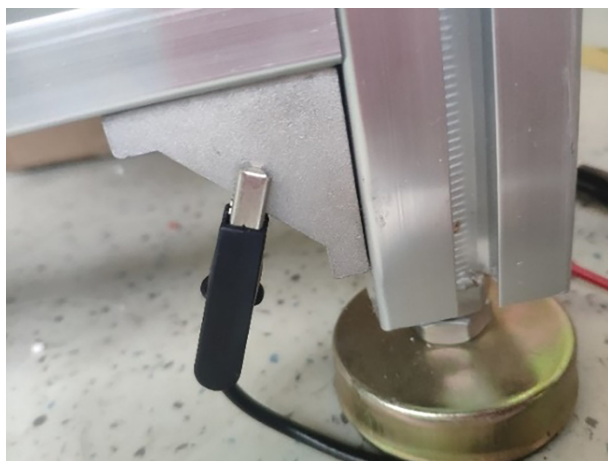
Fig. 5 Grounding the experimental platform.
