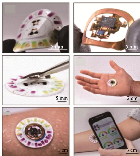
**Fig.4 A Battery Free Wireless Electronic Sensing Platform** <sup>[67]</sup>
