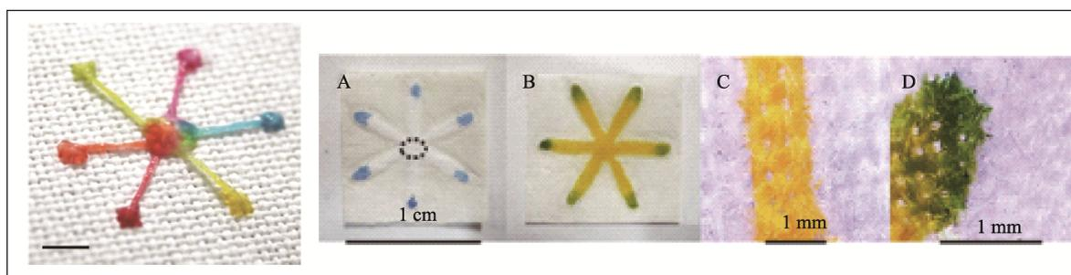
**Fig.3** A Multi-inlet-single-outlet Design Fabricated Using Hydrophilic Cotton Yarn on a Superhydrophobic Textile [36]
