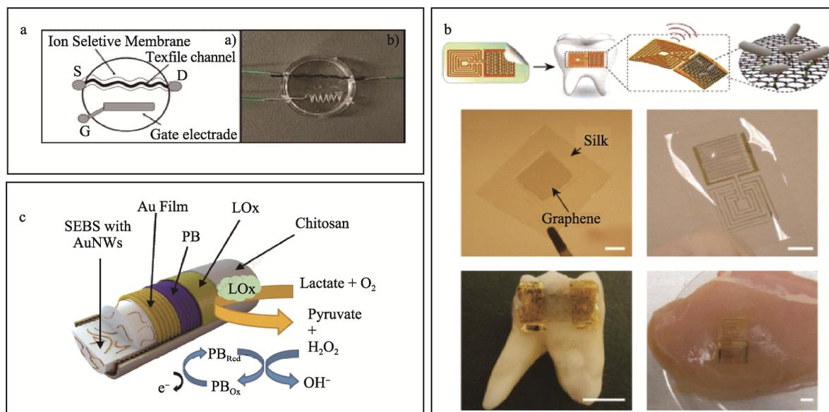
**Fig.2** Textile Integrated Health Monitoring Devices (a) Textile organic electrochemical transistors [70], (b) Dry spun Gold fiber as a Lactate sensitive electrode [60], (c) A schematic and real image of a wireless tattoo-based resistive sensor for *Staphylococcus aureus* [2]
