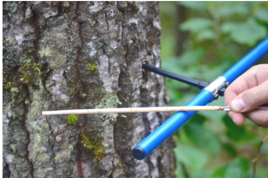
Fig.2 Taking a Sample Using an Increment Borer
