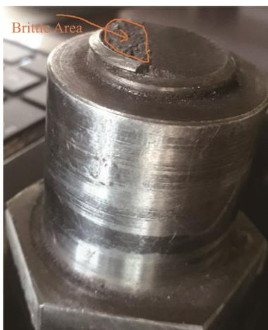
**Fig.6 Brittle Area of the Fracture Surface**
