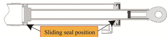
Fig.2 Partial profile of hydraulic actuator seal
