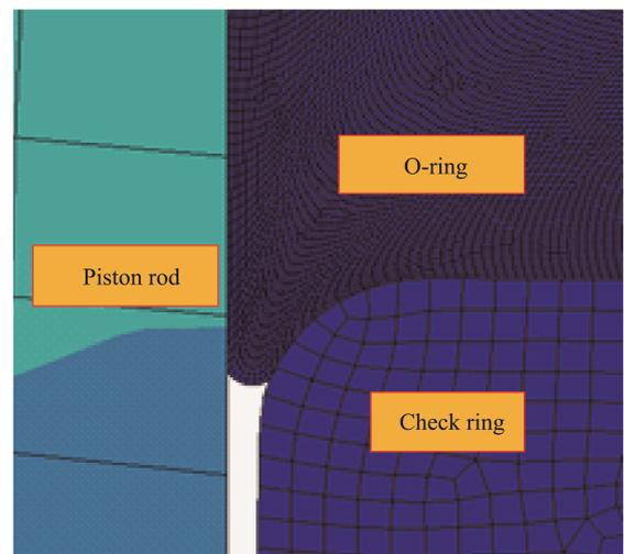
Fig.10 Schematic diagram of O-ring diaphragm
