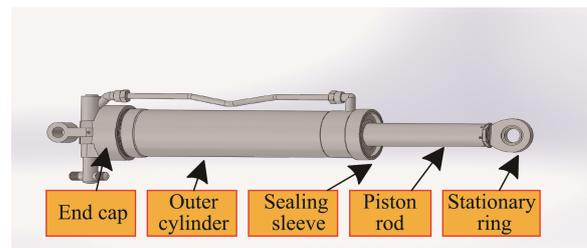
Fig.1 3D model of hydraulic actuator
