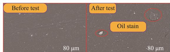
Fig.25 Micro-surface morphology of O-ring
