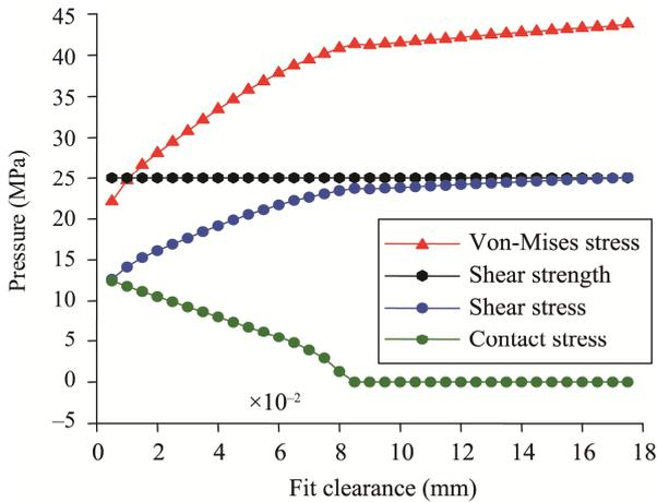
Fig.15 Change curve of check ring stress with fit clearance
