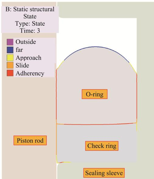
Fig.6 Contact state of each sealing surface
