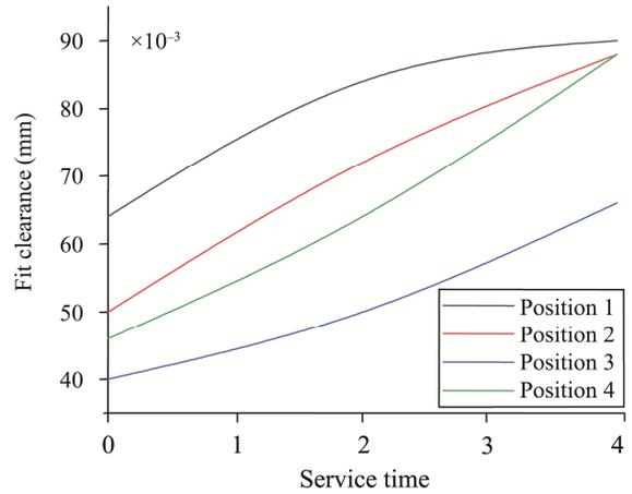
Fig.22 Variation curve of fit clearance with service time
