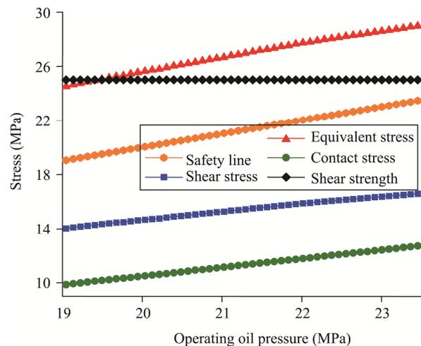
Fig.17 Variation curve of operating oil pressure and check ring stress
