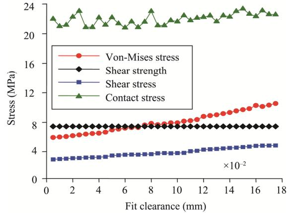
Fig.16 O-ring stress variation curve with fit clearance
