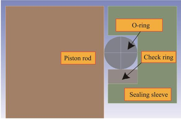
Fig.3 2D axisymmetric model
