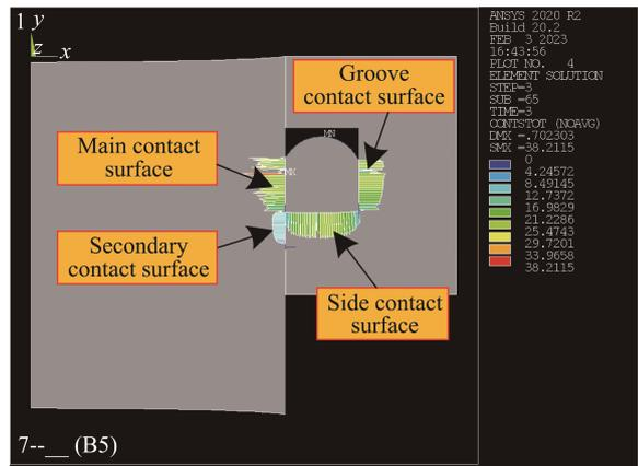
Fig.12 Contact pressure distribution of sealing part after axial compression
