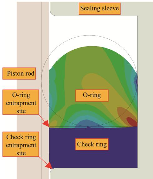
Fig.7 Deformation diagram of sealing assembly under working conditions
