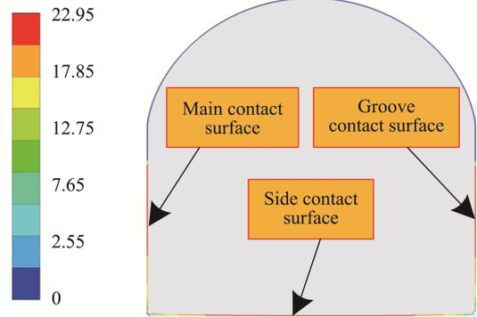
Fig.13 Contact stress distribution diagram of O-ring
