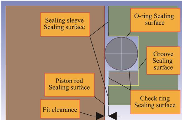
Fig.4 Schematic diagram of sealing two-dimensional contact surface
