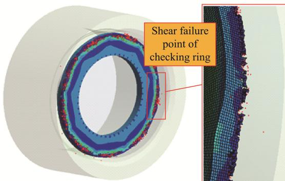
Fig.8 3D diagram of edge damage of check ring
