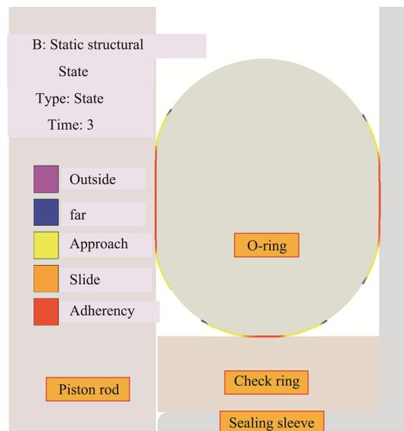
Fig.5 Sealed contact state under precompression
