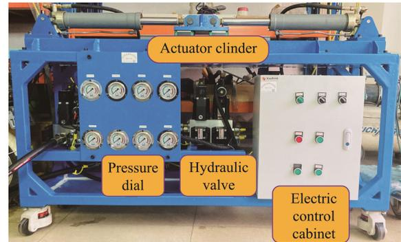
Fig.19 Hydraulic actuator acceleration life test bench
