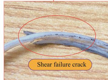
Fig.28 Damaged check ring
