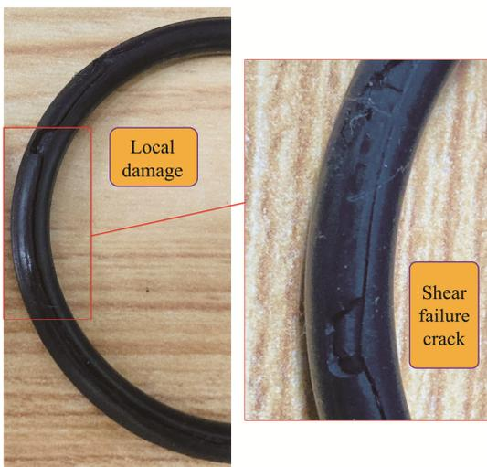
Fig.27 Damaged O-ring
