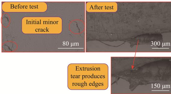
Fig.26 Microscopic surface morphology of check ring
