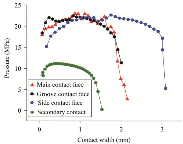
Fig.14 Contact pressure distribution curve of each contact surface of combined seal
