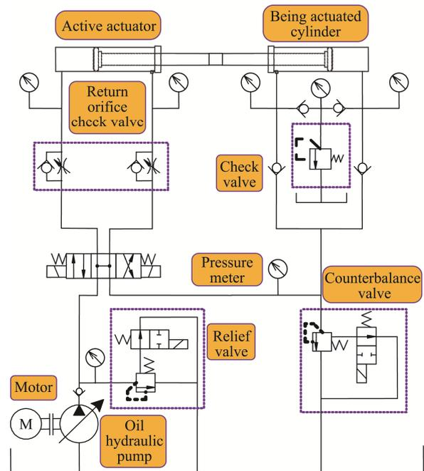
Fig.20 Hydraulic principle of hydraulic actuator acceleration life test bench
