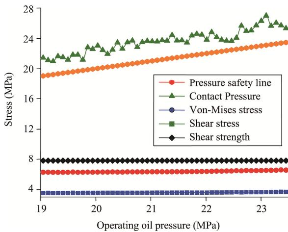
Fig.18 Curve of O-ring stress variation with operating oil pressure
