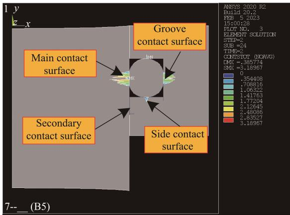
Fig.11 Contact pressure distribution of sealing part after radial precompression
