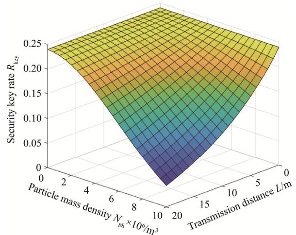
Fig.8 Relationship among security key generation rate, particle number density of marine planktonic algae and transmission distance
