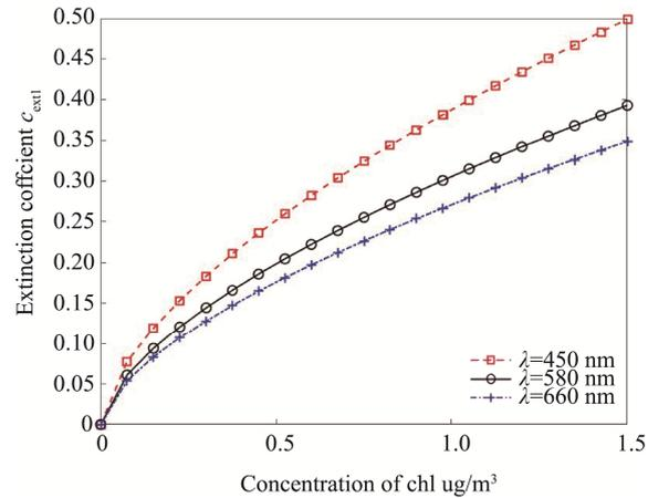
Fig.1 Relationship between chlorophyll concentration and scattering coefficient of algal particles at different wavelengths
