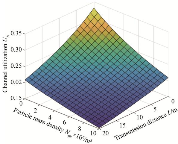
Fig.10 Relationship among channel utilization, particle number density of marine planktonic algae and transmission distance
