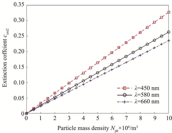
Fig.2 Relationship between particle density and extinction coefficient of planktonic algae at different wavelengths
