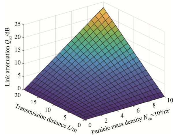
Fig.4 Relationship among link attenuation, particle number density of marine planktonic algae and transmission distance
