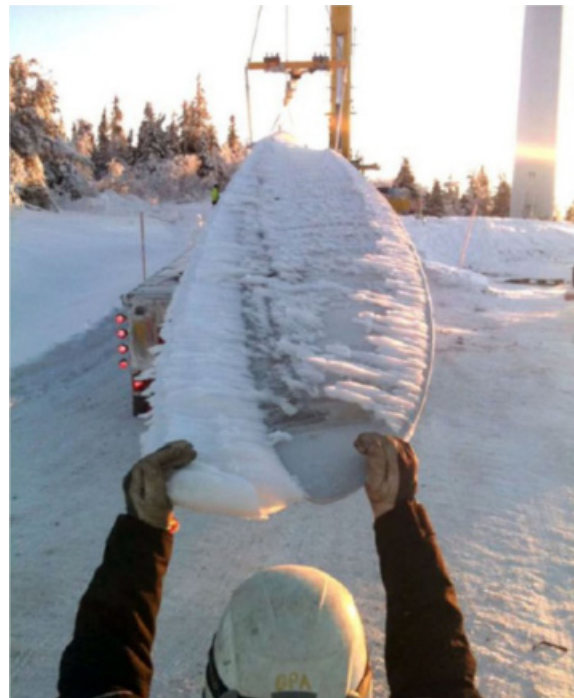
Fig.4 Ice Accretion on a Turbine Blade
