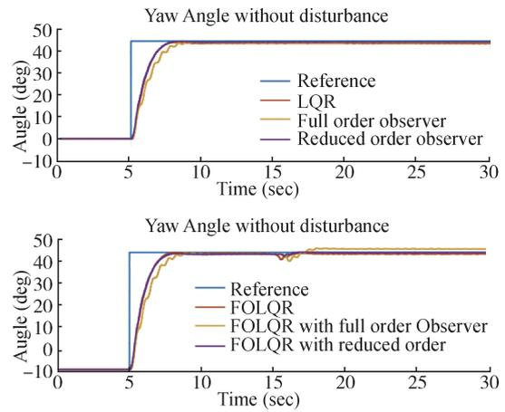
Fig.13 Yaw Stabilization with and without disturbances
