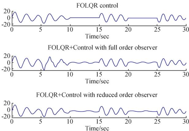
Fig.9 Motor Input (Yaw)
