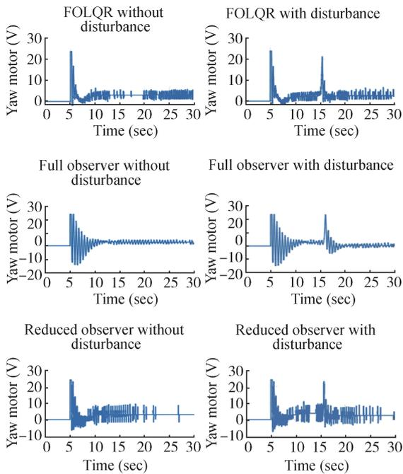
Fig.15 Response related Yaw Motor Input for Stabilization
