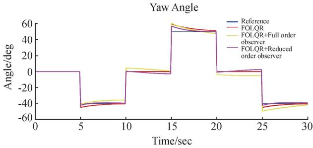
Fig.7 Yaw tracking using FOLQR, FOLQR with full order observer and reduced order observer design
