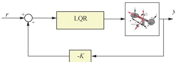
Fig.4 Simple Block Diagram for LQR Control
