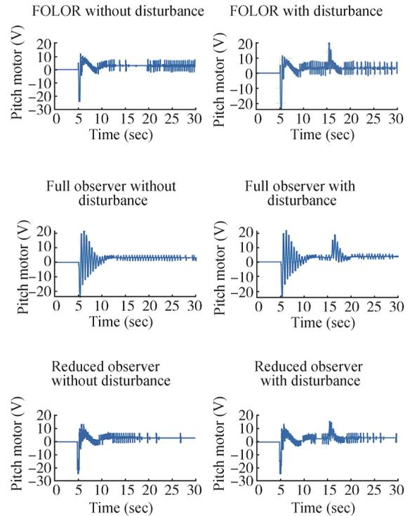
Fig.14 Response related Pitch Motor Input for Stabilization
