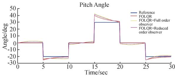
Fig.6 Pitch tracking using FOLQR, FOLQR with full order observer and reduced order observer design
