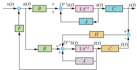
Fig.5 Block Diagram of FOLQR with Observer Design
