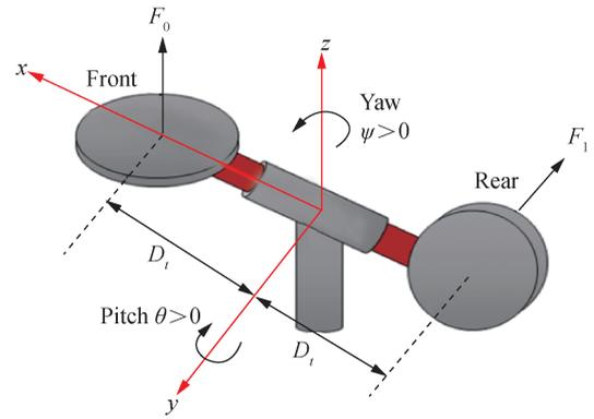
Fig.3 Aero 2-Free body Diagram (Quanser)
