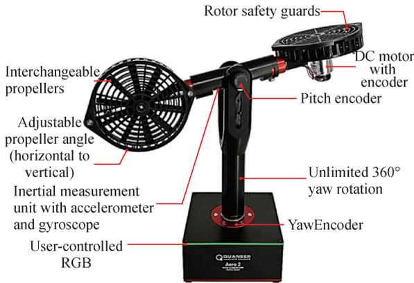
Fig.2 Aero 2 Helicopter Physical System (Quanser)
