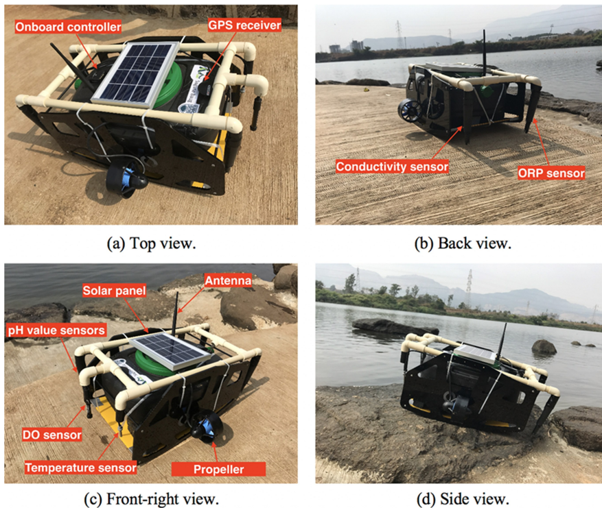
Fig. 6 Mobile sensor node of a water quality monitoring network.
