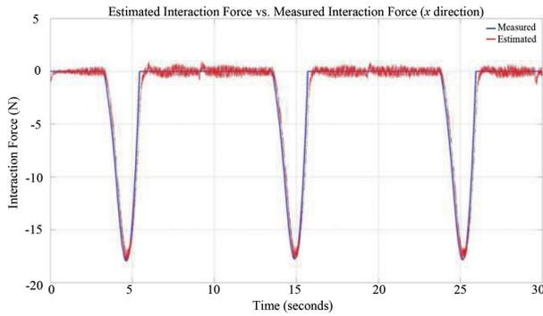
**Fig. 26** Estimated force versus measured force (x direction,  $T_i = 0.1$ ).
