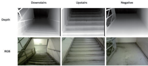
Fig. 4 Different stationary stairways. The first row shows depth images; the second row shows the corresponding RGB images.
