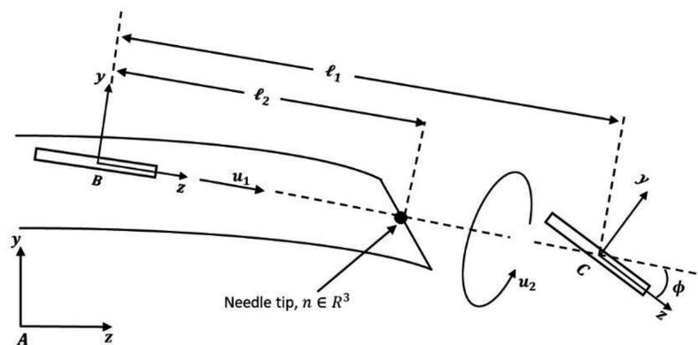
Fig. 1 Configuration of a bevel tip needle during steering showing the front and back wheels at frames  $B$  and  $C$  of a superimposed bicycle-like non-holonomic model<sup>[9]</sup>.
