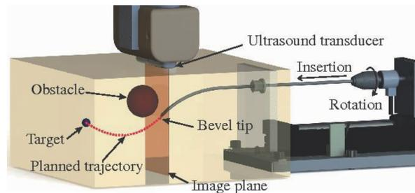
**Fig. 2 A flexible bevel-tip needle is steered inside the tissue phantom by automatic insertion and rotation of the needle base. Using a 2D US transducer, the needle tip pose is estimated for 3D planning [26].**
