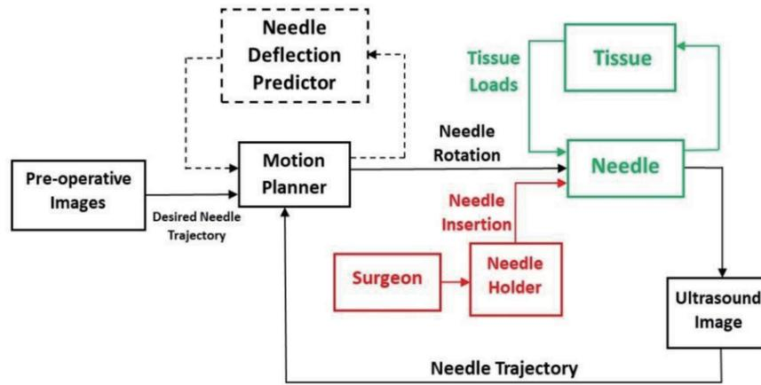
Fig. 5 Block diagram of a closed loop robotic-assisted needle steering system <sup>[38]</sup>.
