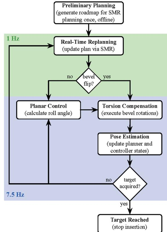
**Fig. 4** Block diagram of an integrated system composed of pose estimator, planner, controller, and torsion compensator <sup>[29]</sup>.
