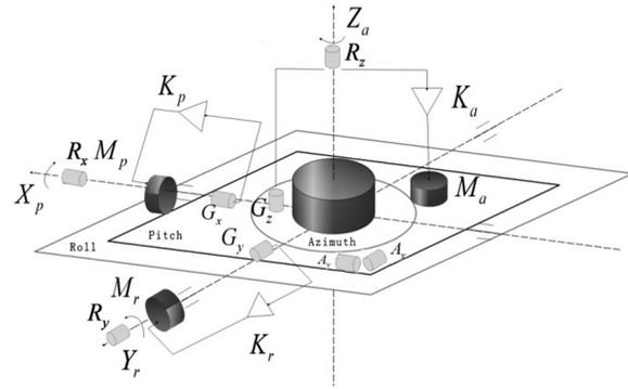
Fig. 1 Schematic diagram of three-axis inertial stabilization platform system.
