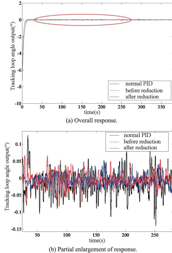
**Fig. 8 Contrast diagram of dynamic pedestal leveling of robust  $H^\infty$  loop shaping platform before and after reduced-order and PID control.**
