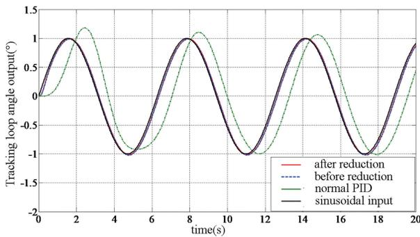
**Fig. 6 Contrast diagram of robust  $H^\infty$  loop shaping controller before and after reduced-order of tracking loop sinusoidal response and PID control.**
