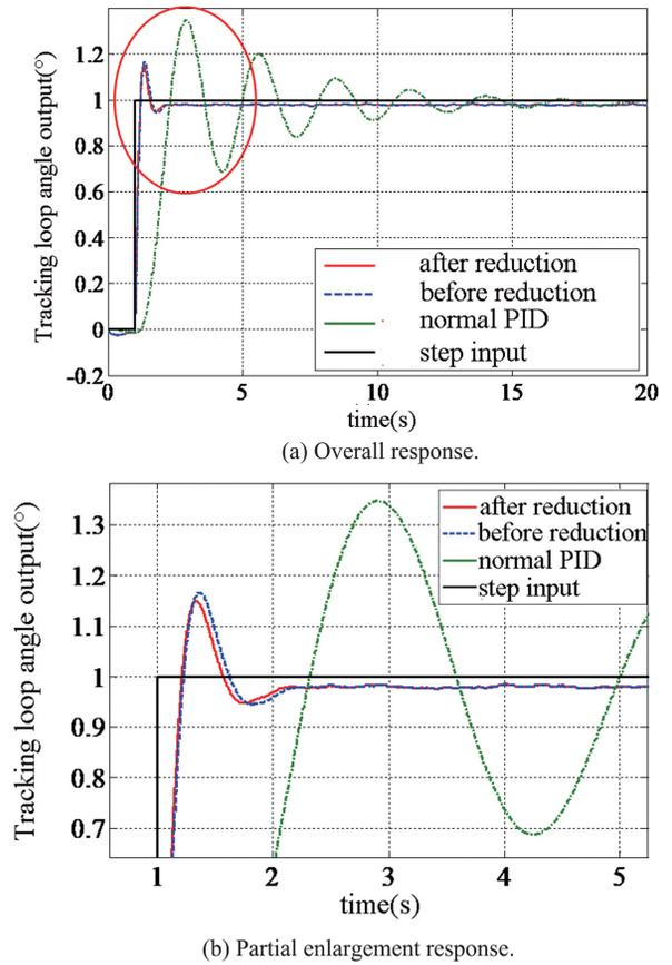
**Fig. 5 Contrast diagram of robust  $H^\infty$  loop shaping controller before and after reduced-order of tracking loop step response and PID controller.**
