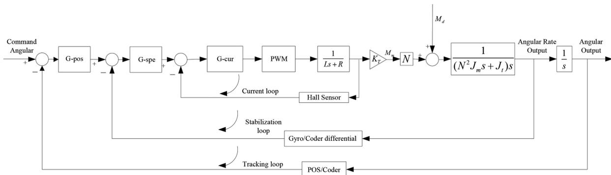
Fig. 2 A block diagram of traditional three-loop control system for ISP.
