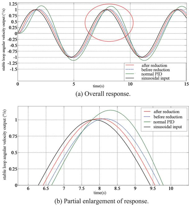
**Fig. 4 Contrast diagram of robust  $H^\infty$  loop shaping controller before and after reduced-order of stable loop sinusoidal response and PID control.**
