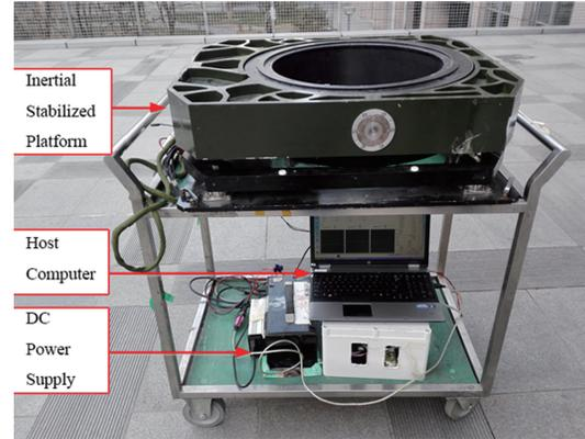
**Fig. 7 Robust  $H^\infty$  loop shaping control platform diagram with moving base.**
