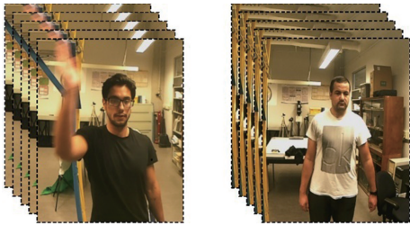
Fig. 8 Sample cropped persons images: Left image shows a detected person performing the "Swiping Hand Left" gesture (used as Park IN trigger). Right image shows a detected person not performing any hand gesture. Both outputs consist of 30 frames each and are both passed to the 3D-CNN gesture recognition network.
